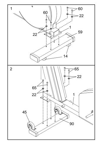
2. Attach the Front Stabilizer (90) to the Frame (1) with the four M10 x 43mm Screws (65) and four M10 Split Washers (22). Make sure that the Front Stabilizer is turned so the Wheels (45) are not touching the floor.
